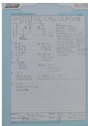
Figure 13. & Figure 14. Shooter Speed Calculation
