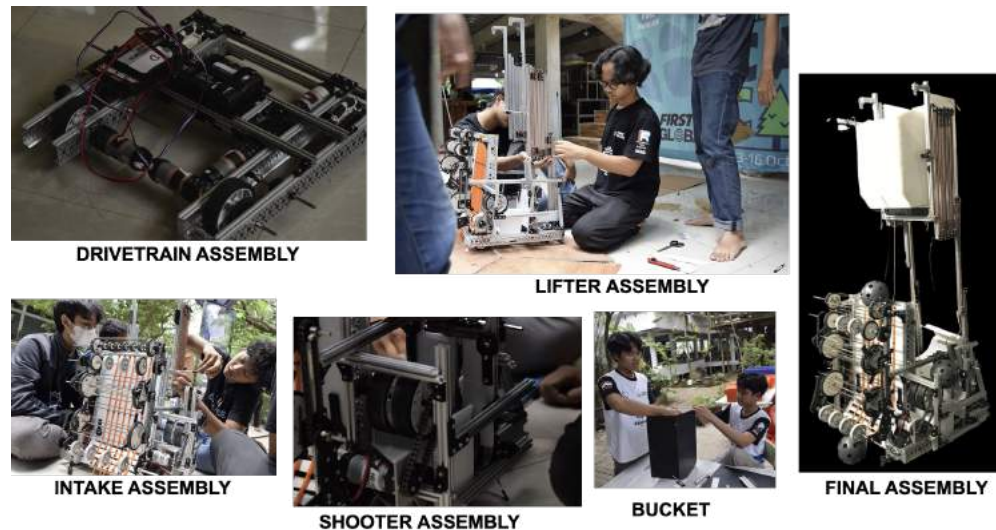
Figure 21. Part prototyping and assembly of Carbon Capture robot
