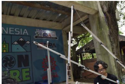
Figure 25. The broken and fallen down lifter structure
